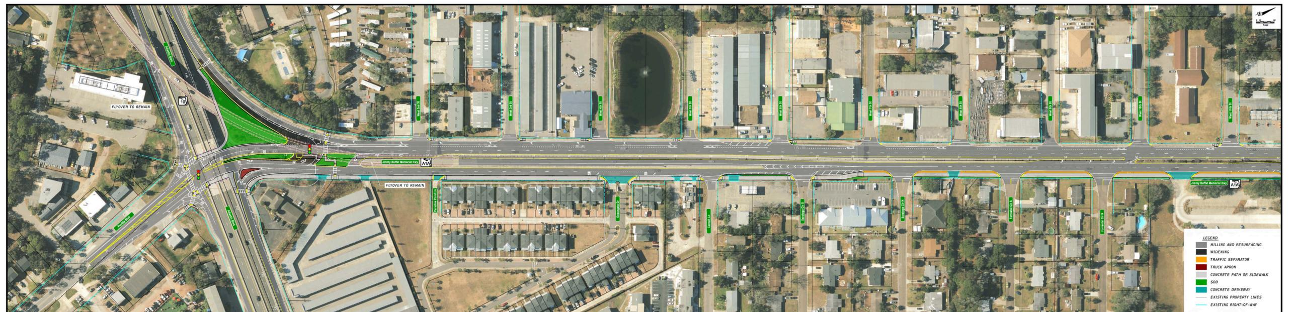
The above rendering represents the milling and resurfacing, upgraded signalized intersection improvements, lane repurposing, southbound bike lane construction and northbound sidewalk widening on Mayport Road (State Road A1A) from Atlantic Boulevard (State Road 10) to Dutton Island Road West.
